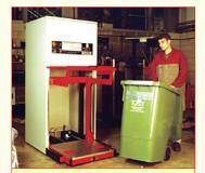
Simply wheel the bin onto the machine ensuring the lid is open, & pull down locating arm.
