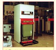
The bin is drawn into the machine, waste is compacted and the bin is automatically returned for reloading.
