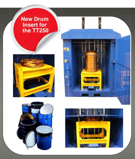
The New Drum insert for the **Tony Team TT250 Baler** is a great optional extra for compacting smaller oil barrels (25 litre to 100 litre) and other small to medium metal containers.
