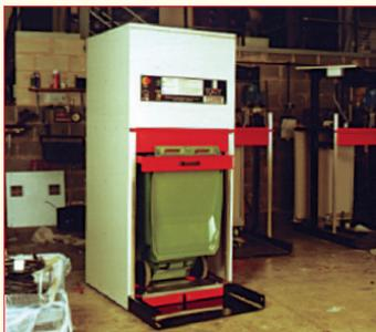
3. The bin is drawn into the machine, waste is compacted and the bin is automatically returned for reloading.
