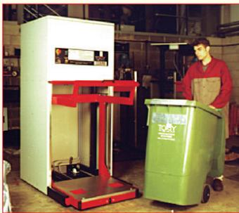
1. Simply wheel the bin onto the machine ensuring the lid is open, & pull down locating arm.
