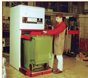
4. Orange light indicates bin is full. Simply remove bin & replace with an empty one.
