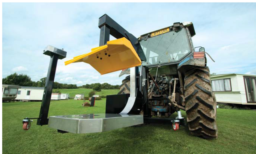
Bin compactor with tractor attachment
